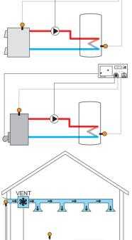
DTC 200/2G is a differential thermostat, designed for heating DHWT (domestic hot water tank) from one heating source (solar collectors, boilers, heat pumps) with possibility to control the burner or electric heater.
