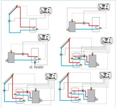
DTC 100/4 TD is a differential digital thermostat, designed for heating DHWT (domestic hot water tank) from two heating sources (solar collectors, boilers, heat pumps) and for controlling the burner or electric heater.
