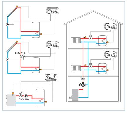
DTC 100/2 is a differential thermostat, designed for heating DHWT (domestic hot water tank) from one heating sources (solar collectors, boilers, heat pumps).
