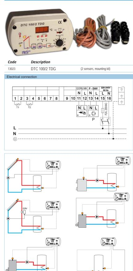
DTC 100/2 TDG is a differential digital thermostat, designed for heating DHWT (domestic hot water tank) from one heating source (solar collectors, boilers, heat pumps) with possibility to control the burner, or electric heater.
