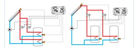
DTC 100/3 is a differential thermostat, designed for heating DHWT (domestic hot water tank) with two storage tanks from one heating source (solar collectors, boilers, heat pumps). It is used in the systems where during the day one storage tank cannot accumulate whole energy, which is disposal from solar collector.
