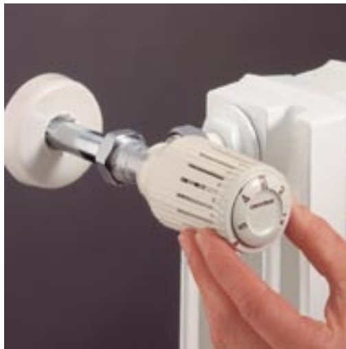
Attach the thermostatic head to the valve. Ensure that the half moon recesses on the base of the head align with the protruding lugs on the body.
