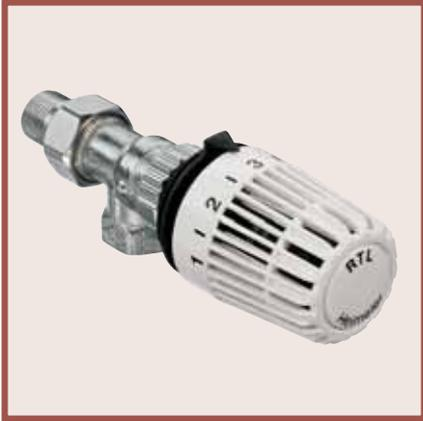
The HEIMEIER return temperature limiter RTL is an automatic thermostatic controller. The temperature of the flowing medium is transferred to the sensor via conductivity. This keeps the specified value constant within a proportional band necessary for control. The valve only opens when the set limiting value has not been reached.
