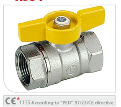
DADO® ball valve, nickel plated, female connections and T handle. Full port. Heavy-type series.
