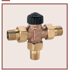
HEIMEIER three-way mixing valve, with or without presetting, for mixing volume flows in heating and cooling systems, made of gunmetal, with protection cap.
